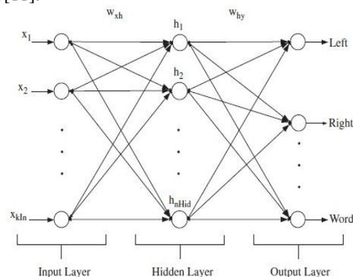
Fig 3:Three-layer feed-forward neural network
